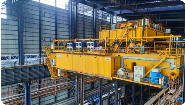
Supply of Powerform & Hyflex ropes to one of the largest E.O.T cranes manufactured in China. Six units of these E.O.T cranes, each with a lifting capacity of 550 metric tonnes, have been installed in one of India's leading steel plants.
